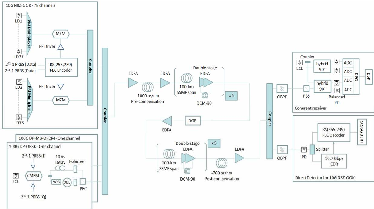
**Fig. 2:** Set-up of the 124.4 Gbps DP-MB-OFDM, 112 Gbps DP-QPSK, 10.7 Gbps NRZ-OOK transmitters, 10x100 km G.652 fiber transmission line, coherent receiver and direct detector with PM (polarization-maintaining), PBS (polarization beam splitter), ADC (analog-to-digital converter), RS (Reed-Solomon), PD (Photodiode).
