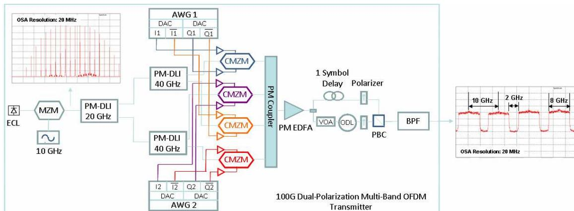
**Fig. 1:** Set-up of the 124 Gbps DP-MB-OFDM transmitter with PBC (polarization beam combiner), ODL (optical delay line), VOA (variable optical attenuator). In insets are represented the spectrum of the 10-GHz-spaced optical carriers at the MZM output, and the spectrum of the 124 Gbps DP-MB-OFDM signal at the transmitter output.
