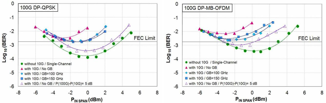
**Fig. 3:** BER versus span input power per channel after the dispersion-managed 10x100-km G.652 fiber line for the 112 Gbps DP-QPSK and the 124 Gbps DP-MB-OFDM signals for the various configurations under study.
