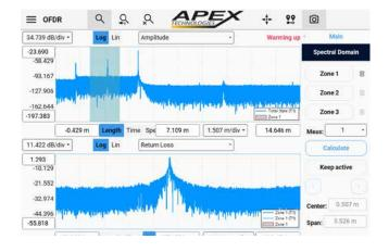
Analyze the insertion losses and return losses in time domain *and* spectral domain
