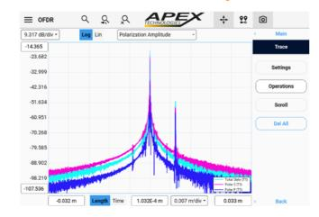
Two (2) orthogonal polarization states are measured independantly and displayed, individually or combined
