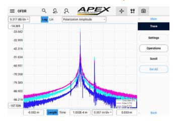
Two (2) orthogonal polarization states are measured independantly and displayed, individually or combined
