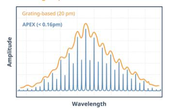
Hundreds of times better resolution than grating-based/monochromator OSA allows to accurately measure the smallest features.
