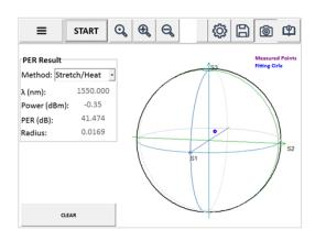
SOP, DOP, and PER measured with high accuracy and allowing fast sampling rates, over a wide range of input optical power. Information displayed as Jones vectors, Poincare sphere, and Stokes parameters.
